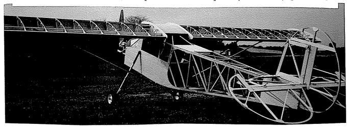
Wings fold for storage. Ailerons will remain installed but flaps will need to be removed with quick release pins. (2 mins.)
